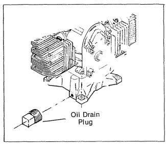
1. With engine still warm from running, remove Oil Drain Plug at base of engine. Drain oil completely into a suitable container. Then reinstall Oil Drain Plug securely.
